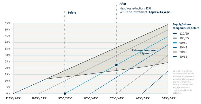
Supply and return temperatures after the mixing point
